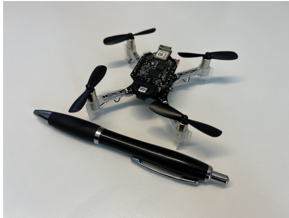
Figure 2.12: A Bitcraze Crazyflie 2.1 with AI deck 1.1 and Flow deck v2 attached.
