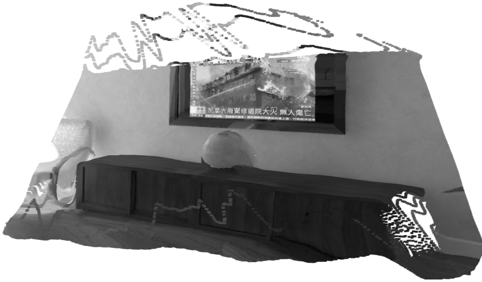
Figure 30: Rendering of reconstructed depth, using depth baseline. The following results were generated for this sample: \lambda : 0.001 | PSNR: 59.35 dB | 0.010 bpp.
