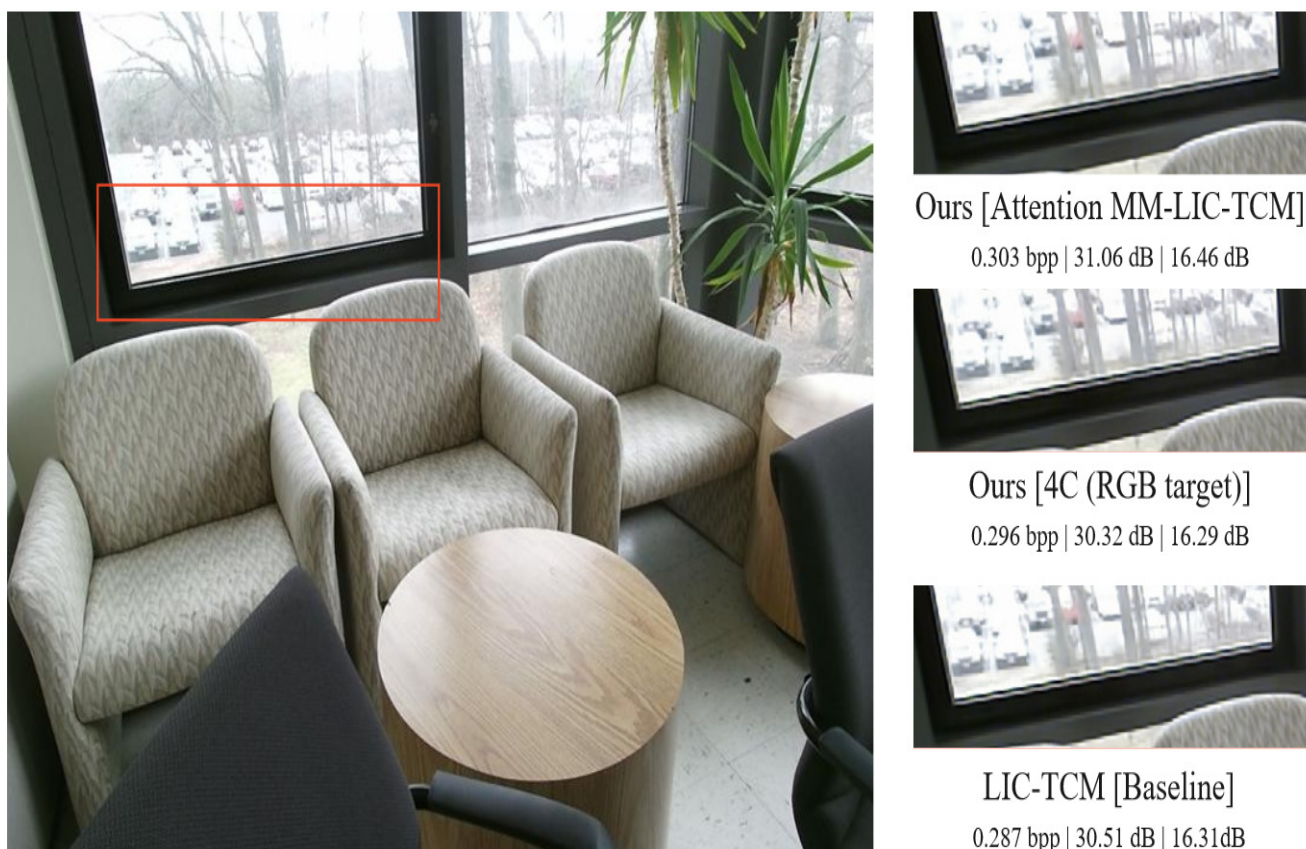
Figure 32: Visualization of decompressed images of frame 0000118, KinectV2, from SUNRGB-D dataset. The large figure to the left is the original image. The subfigures are titled as “Method | Bit rate | PSNR | MS-SSIM”.
