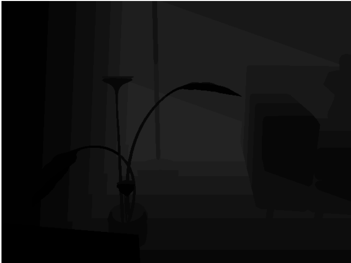
Figure 8: An example of the typical representation of a depth image. Note that the brightness and the contrast of the image are enhanced for better display.
