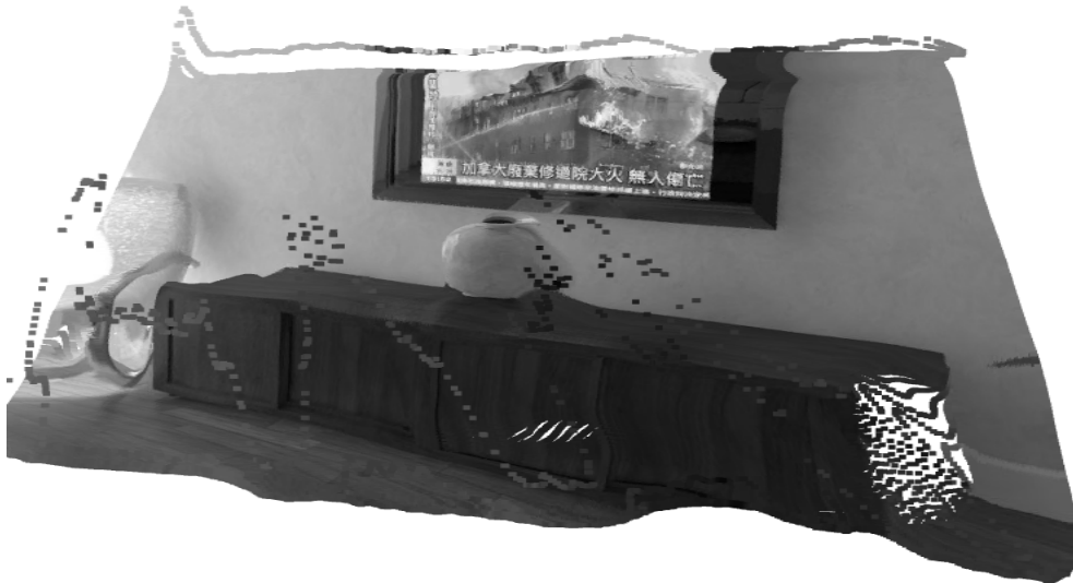
Figure 31: Rendering of reconstructed depth, using Convolutional MM-LIC-TCM architecture. The following results were generated for this sample: \lambda : 0.001 | PSNR: 60.47 dB | 0.020 bpp.
