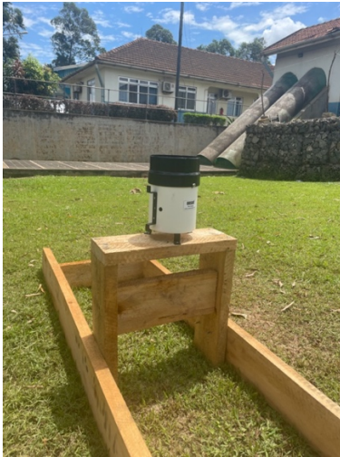
Figure 5 Tipping bucket rain gauge mounted 50 cm above ground.
