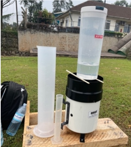
Figure 6 Calibration setup with plastic measuring glasses to the left.
