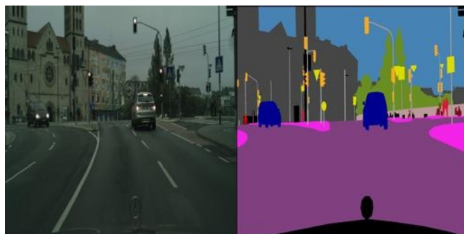
Figure 4: Example image from the dataset Cityscapes[6]. On the right side, colours corresponding to different classes can be seen for each pixel.
