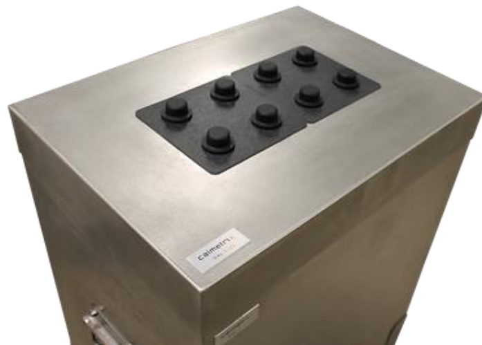
Figure 5. The Calmetrix I-Cal Ultra isothermal calorimeter provides eight channels for individual measurements [33].
