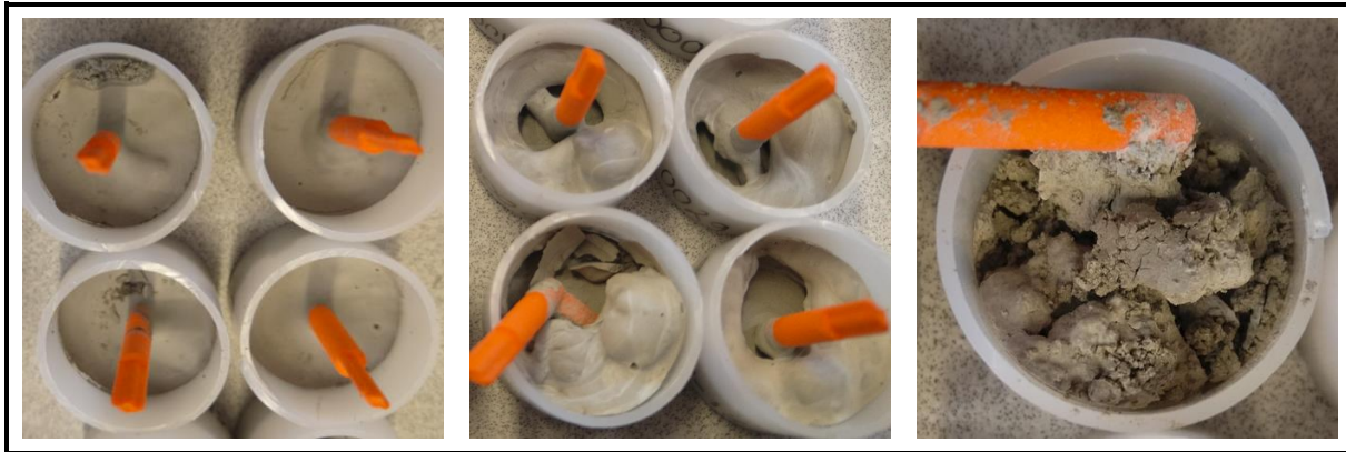
Figure 14. Examples of different mixing qualities achieved through in-situ mixing. To the left are examples of the most homogeneous samples, while the sample to the right was very poorly mixed and not homogeneously hydrated. The middle picture shows intermediate mixing quality, for which it was assumed that the samples were sufficiently hydrated.
