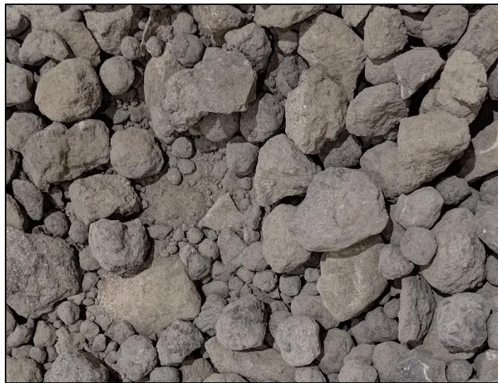
Figure 1. The product leaving the kiln is cement clinker granules of diverse sizes.
