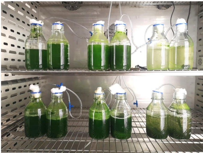
Figure 5: Phase II, day 14. From upper left: 30% AnBW, ref: Z8, and ref: no algae (contaminated). From lower left: 50% AnBW w/o TE, 50% AnBW w TE, and 50% AnBW unsterilised.
