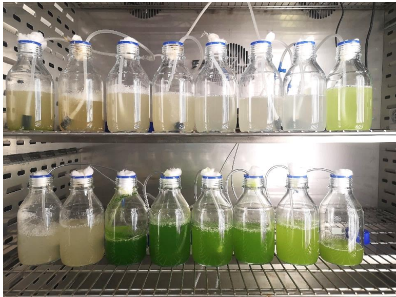
Figure 4: Phase I, day 14. The dilution of AnBW:DI from left to right (in pairs): 100%, 50%, 30%, and 10%. The bottles at the lower row are enriched with CO 2 .
