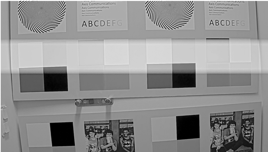
Figure 2.7: Shows a strobe artefact in the form of a bright band across the image.
