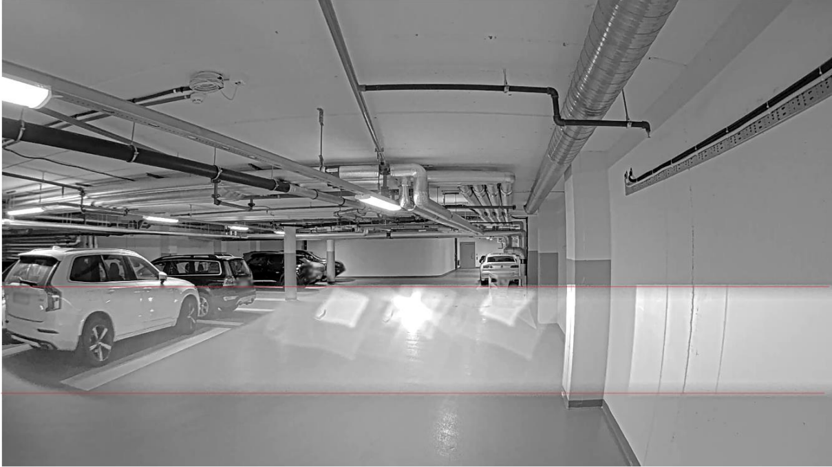
Figure 4.19: Shows the strobe 10 m away, pointed at the camera. Note the concentration of the light.
