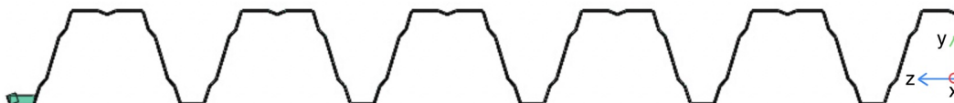
Figure 4.9: Thickness of roof scaled 3 times thicker than actual width, where the edge is 5 mm and remaining 0.8 mm.
