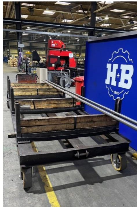
Figure 27: Chassis on castors inside of the warehouse of Heine + Beisswenger.
