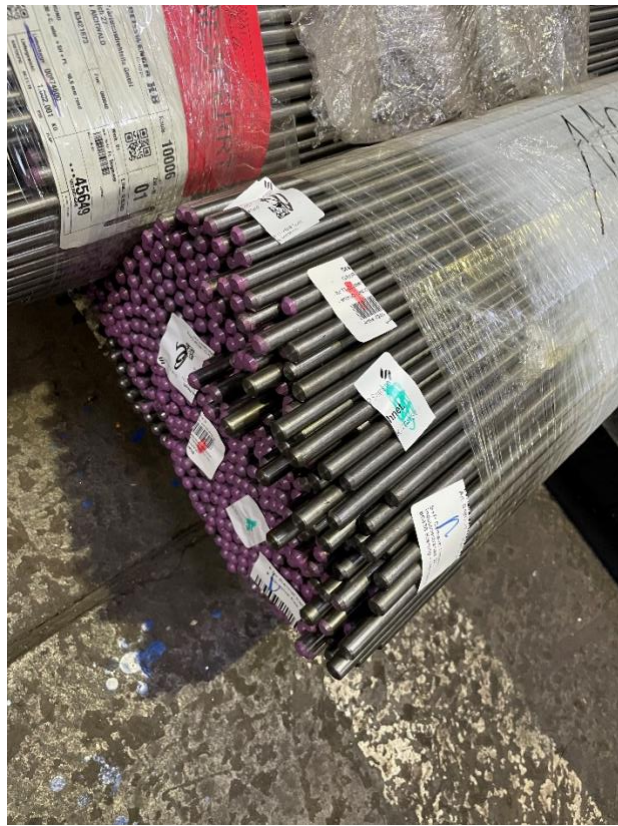
Figure 24: Round steel bars tied into a bundle.
