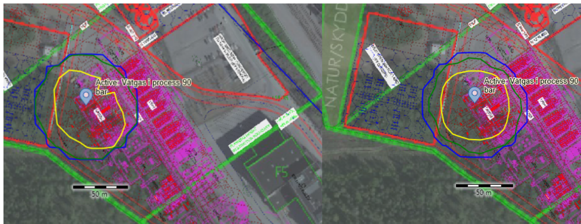
Figure 7.1: Risk contours generated from iteration 1 (left and the original assessment (right)). Yellow: 1E-7 /year, Green: 1E-8 /year, Blue: 1E-9 /year.
