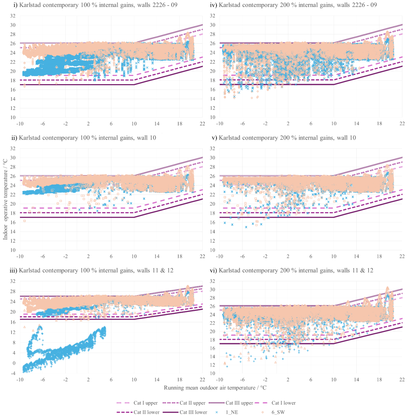
Figure 30. Indoor operative temperature in relation to the outdoor running mean temperature. Hourly zone data for the contemporary climate of Karlstad at 100 % (left) and 200 % (right) of internal gains are plotted for different wall assemblies, with marked limits of the thermal comfort categories I – III, according to the EN 16798-1:2019 standard.
