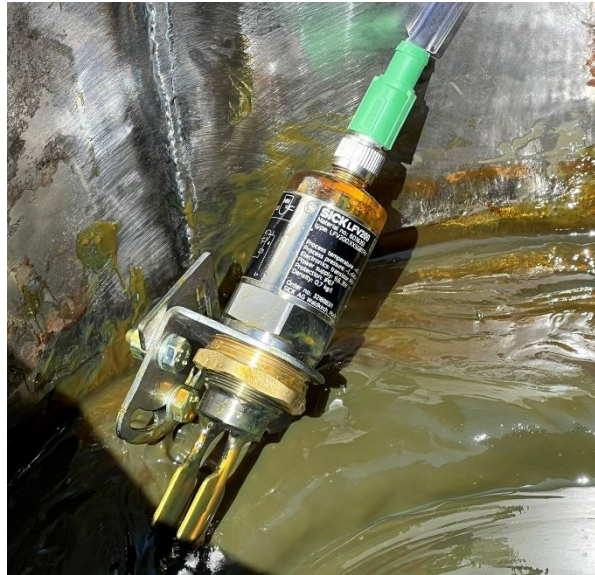
Figure 7.2 Picture of the mounting position of the LFB200 from test eleven.
