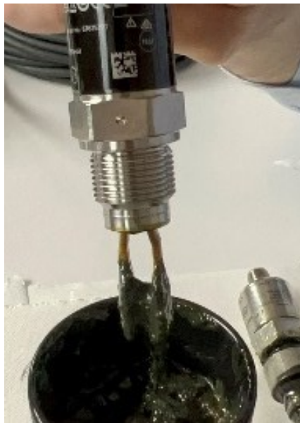
Figure 5.11 Buildup of dirty grease on LFV200.
