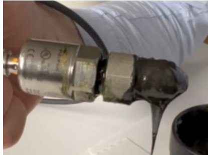
Figure 5.10 Buildup of grease with metal particles on LMT110.
