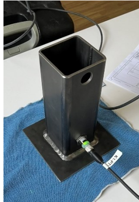
Figure 5.4 Steel profile for testing.
