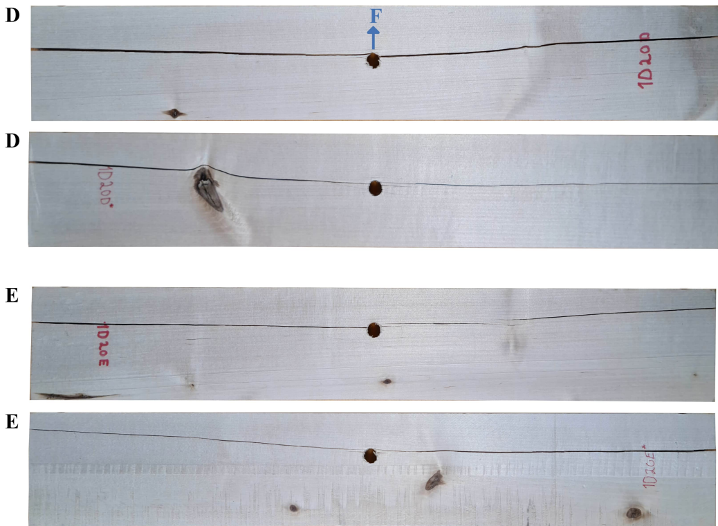
Figure 7.12: Beam 1D20D and 1D20E after the dowel tests.
