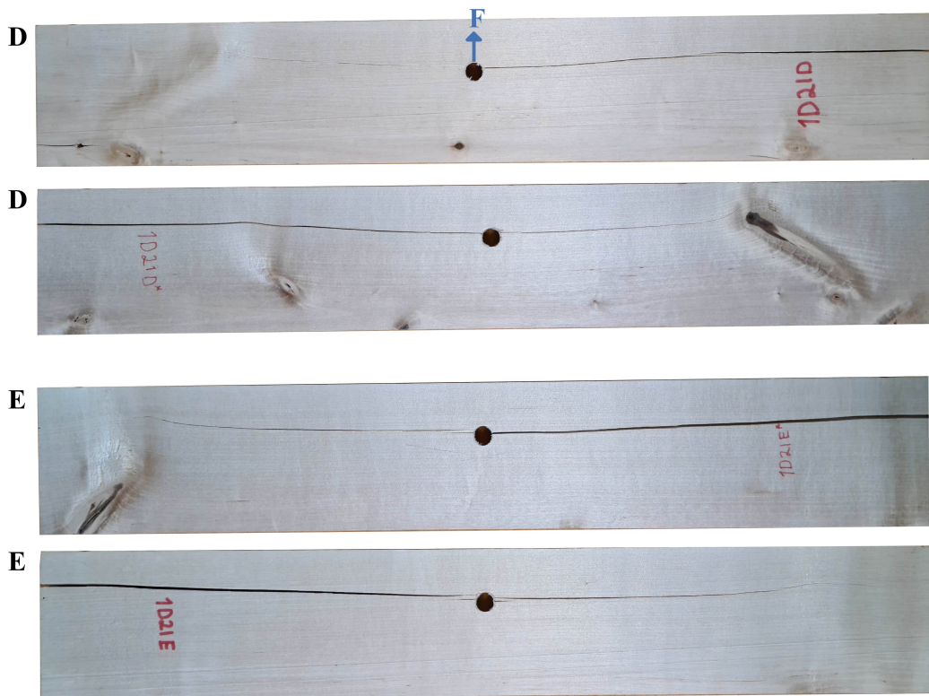
Figure 7.14: Beam 1D21D and 1D21E after the dowel tests.
