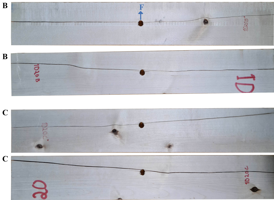
Figure 7.11: Beam 1D20B and 1D20C after the dowel tests.
