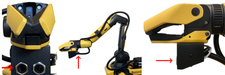
Figure 4.1 Camera placement on Spot.
