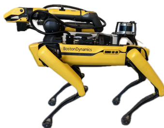
Figure 2.1 The quadruped autonomous mobile robot Spot developed by Boston Dynamics.
