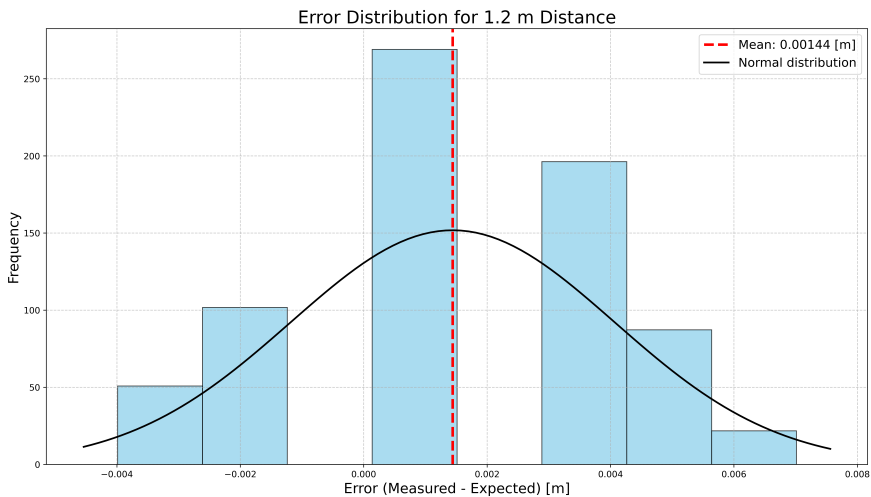
Figure 5.3 Distribution of errors at a distance of 1.2 m, with the mean value highlighted and featuring the distribution curve.
