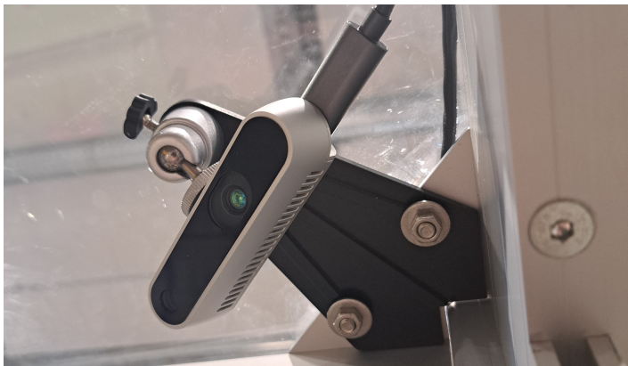
Figure 3.4 The Intel RealSense D435i depth camera with mounting bracket inside the robot cage.
