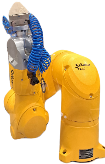
Figure 3.1 The Staubli TX60 industrial robot with pneumatic gripper.
