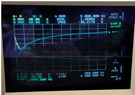
Figure 44: On the left, impedance measurements of two speaker drivers in parallel. On the right, impedance measurements of two speaker drivers in series. Yellow line shows the real part of the impedance and blue line shows the imaginary part of the impedance.
