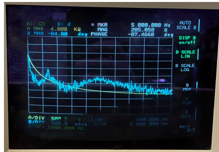
Figure 42: On the left, impedance measurements of four speaker drivers in parallel. On the right, impedance measurements of four speaker drivers in series. Yellow line shows the magnitude of the impedance and blue shows the phase.
