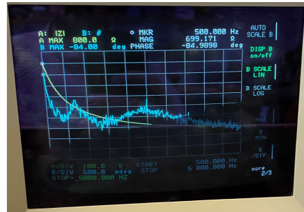
Figure 39: On the left, impedance measurements of one speaker driver. On the right, impedance measurements of four speaker driver connected as a parallel connection between two sets of series connections. Yellow line shows the magnitude of the impedance and blue shows the phase.
