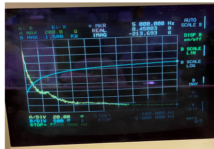
Figure 45: On the left, impedance measurements of three speaker drivers in parallel. On the right, impedance measurements of three speaker drivers in series. Yellow line shows the real part of the impedance and blue line shows the imaginary part of the impedance.
