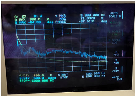
Figure 39: On the left, impedance measurements of one speaker driver. On the right, impedance measurements of four speaker driver connected as a parallel connection between two sets of series connections. Yellow line shows the magnitude of the impedance and blue shows the phase.
