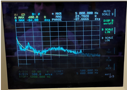
Figure 41: On the left, impedance measurements of three speaker drivers in parallel. On the right, impedance measurements of three speaker drivers in series. Yellow line shows the magnitude of the impedance and blue shows the phase.
