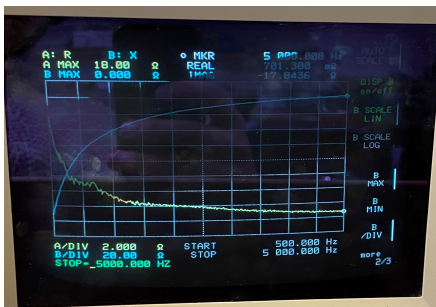
Figure 46: On the left, impedance measurements of four speaker drivers in parallel. On the right, impedance measurements of four speaker drivers in series. Yellow line shows the real part of the impedance and blue line shows the imaginary part of the impedance.
