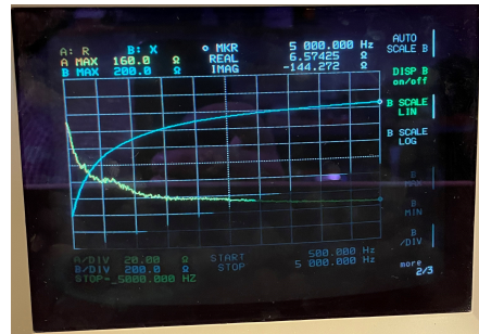
Figure 44: On the left, impedance measurements of two speaker drivers in parallel. On the right, impedance measurements of two speaker drivers in series. Yellow line shows the real part of the impedance and blue line shows the imaginary part of the impedance.
