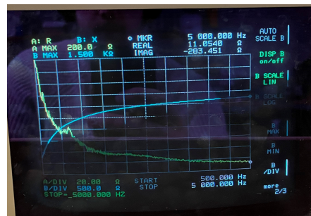
Figure 46: On the left, impedance measurements of four speaker drivers in parallel. On the right, impedance measurements of four speaker drivers in series. Yellow line shows the real part of the impedance and blue line shows the imaginary part of the impedance.
