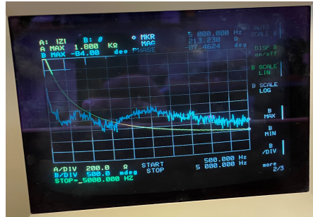
Figure 41: On the left, impedance measurements of three speaker drivers in parallel. On the right, impedance measurements of three speaker drivers in series. Yellow line shows the magnitude of the impedance and blue shows the phase.
