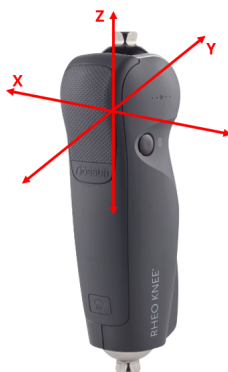
Figure 3.2 Rheo Knee 3 - The figure showcases the orientation of the three-dimensional axis with respect to the knee.
