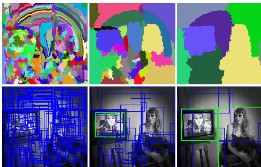
Figure 2.3 An illustration of Selective Search algorithm at different iteration. There are four types of similarities considered in the algorithm: color, texture, size, and fill. The bounding boxes (below) are drawn based on the segmented region proposals (above). Figure from [Felzenszwalb and Huttenlocher, 2004]
