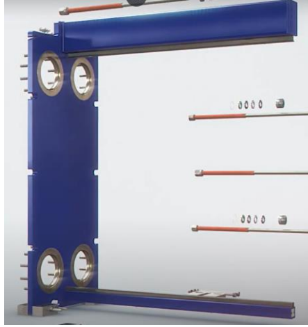
Figure 2.17 Step 3, CB and GB are mounted on the FP (Alfa Laval, 2017).
