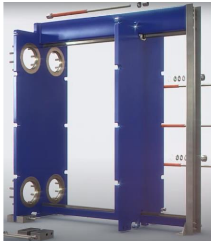
Figure 2.19 Step 5, support column is mounted (Alfa Laval, 2017).
