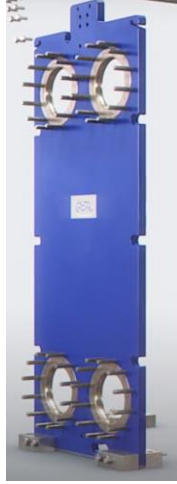
Figure 2.16 Step 2, linings, feet and stud bolts have been placed on the FP (Alfa Laval, 2017).
