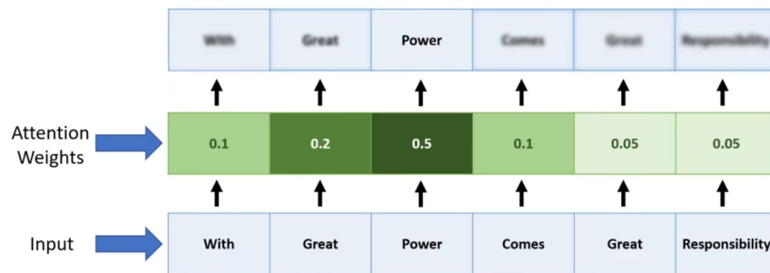
Figure 3.4: The attention mechanism allows a focus on the values. After Halfling Wizard, Attention Mechanism In a nutshell . https://www.youtube.com/watch?v=oMeIDqRguLY
