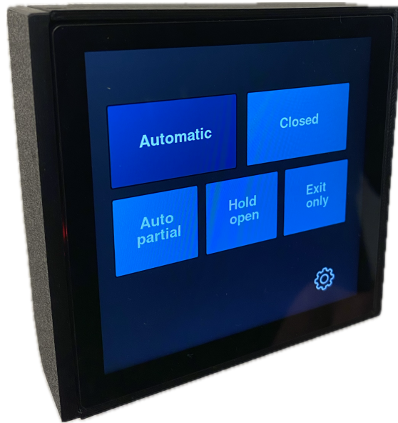
Figure 28: The finished prototype displaying the mode selection menu and the operating modes that can be selected
