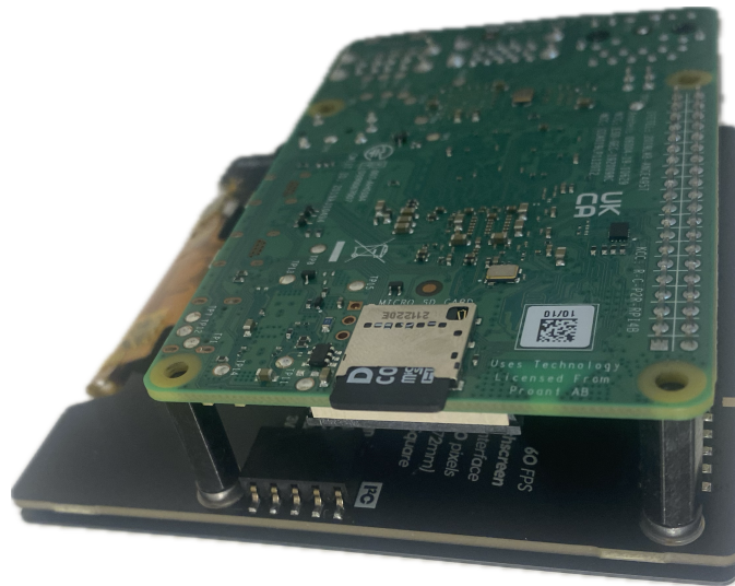
Figure 3: Mounting of display on the Raspberry Pi board.
