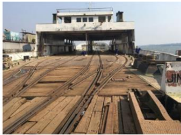
Roll-on / roll-off ferry with railway tracks
