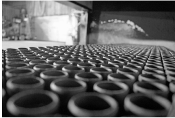
Figure 16 - Flame suppressing lattice used in SP Fire 105 test [59].
