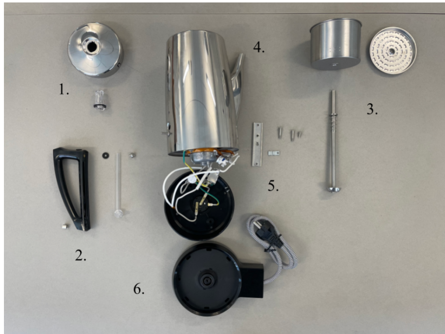
Figure 3.1: The current percolator model from C3 when disassembled.
