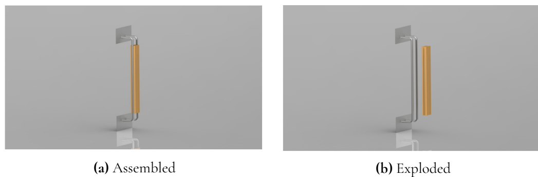
Figure 5.2: Non-screwed on wooden handle
