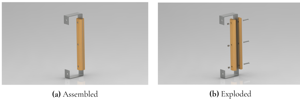
Figure 5.1: Screwed on wooden handle
