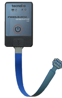
Figure 2. Tecnia multichannel generator connected to a 16-electrode multipad.
