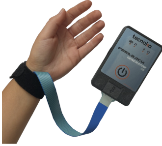
Figure 3. Placement of the multipad electrode on the participants wrist, held in place by an elastic strap.
