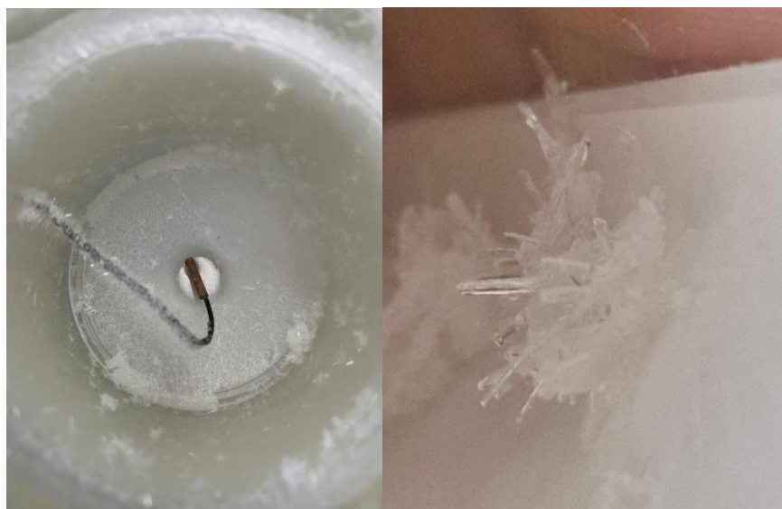
Figure 4.12. Crystallization on the inner walls of the reactor
