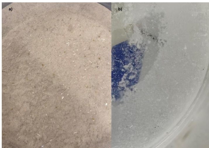
Figure 4.11. Crystallization at the bottom of the reactor: a) crystals after filtration, b) crystals at the bottom of the setup
