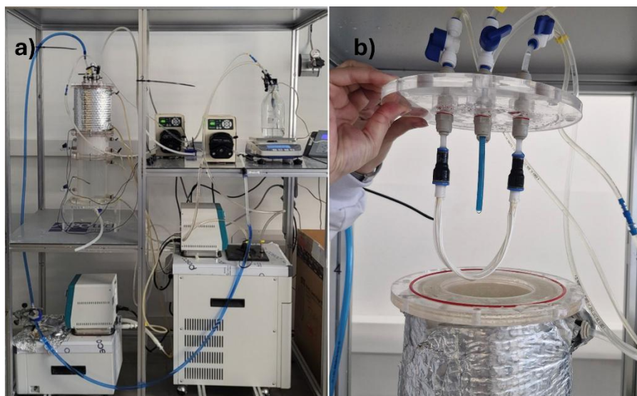
Figure 3.1. a) Setup including the reactor, pumps, scale, conductivity meter, heater, and cooler b) Hollow fiber membrane hanging from the top section of the reactor
