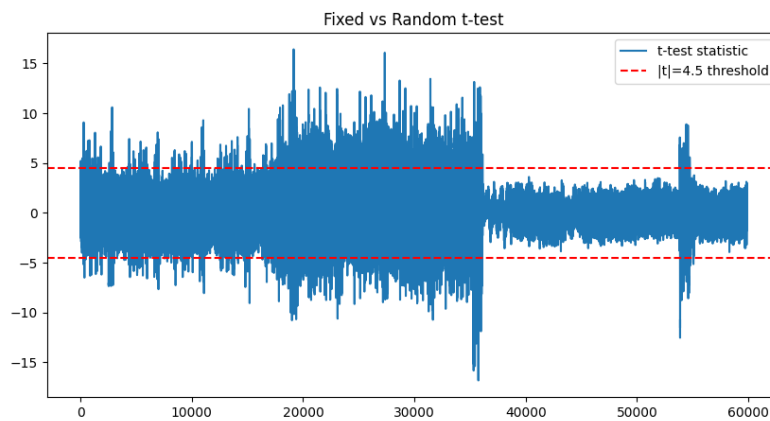
Figure 4.4: The t-test between the groups m = 0 vs m = rand() to see if pointwise difference in mean exists in the power traces. The threshold was set to 4.5. 4143 of 60k points (6.905%) had |t| \geq 4.5
