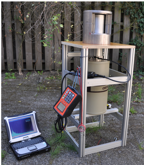
Figure 9: Collimator and detector mounted in the aluminium rack.
