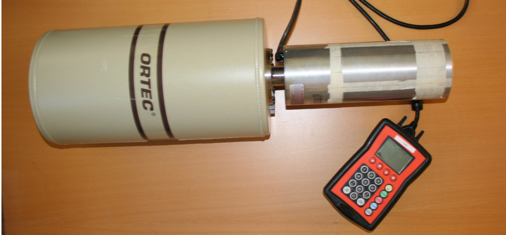
Figure 4: The HPGe-detector connected to DigiDART.
