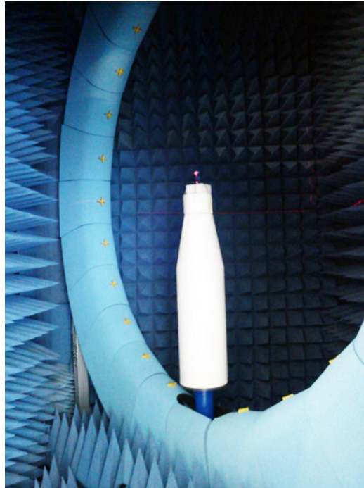
Figure 15: A spherical near-field antenna test range (SNFT). The antenna under test (AUT) is positioned on the rotating stand in the middle, and the measurement probes are mounted in an arch. A laser pointer is used to position the antenna accurately. The walls, floor and ceiling of the anechoic chamber are covered with radiation absorbent material. The photograph was taken when the Skycross ultra-wideband (UWB) antenna in Figure 2d in Paper V was characterized in a Satimo Stargate-24 chamber at Lite-On Mobile, Lund, Sweden. The author thanks Anders Sunesson for permission to use the photograph.
