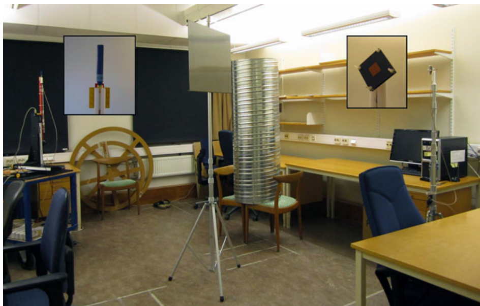
Figure 3: The measurement scenario, a small room with many scatterers and obstructed-line-of-sight (OLOS). The transmitting patch antenna is mounted on the stand to the right, and the receiving sleeve dipole is mounted on the 3D positioner to the left.
