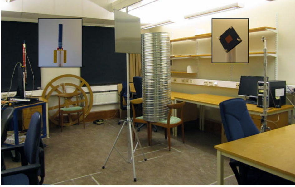
Figure 18: The measurement scenario in Paper V, a small room with many scatterers and obstructed-line-of-sight (OLOS). The transmitting patch antenna is mounted on the stand to the right, and the receiving sleeve dipole is mounted on the 3D positioner to the left.
