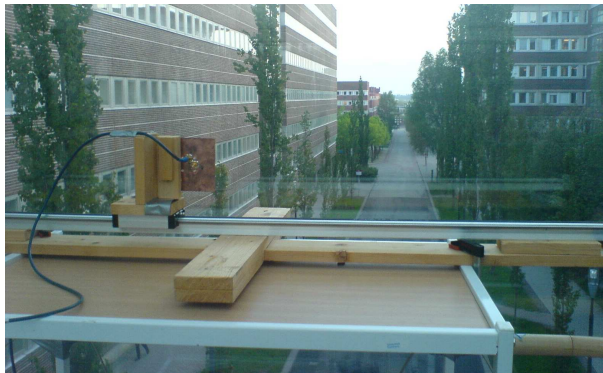
Figure 3.3: Linear positioning robot with TX probe antenna.
