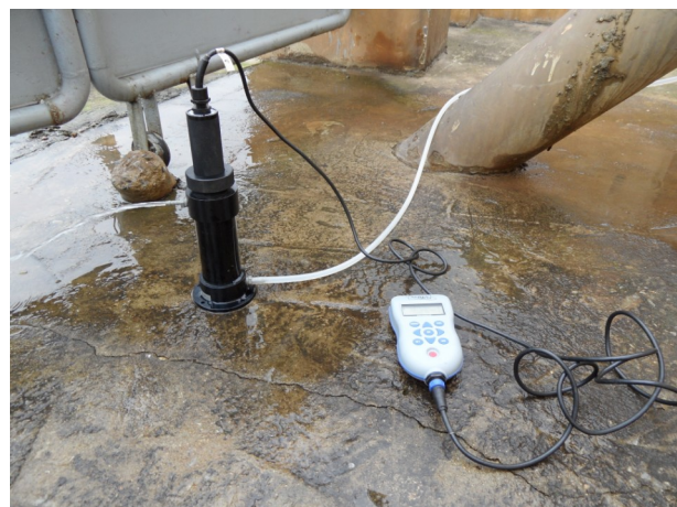
Figure 7. The Aquaread AP-800 Aquameter probe with a flow-through cell.
