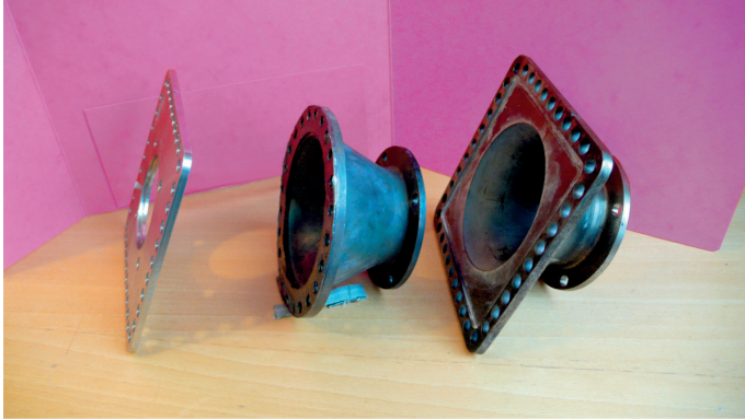
Figure 5.2: Quarl designs. From left to right, flat plate, circular conical expansion and square conical expansion.
