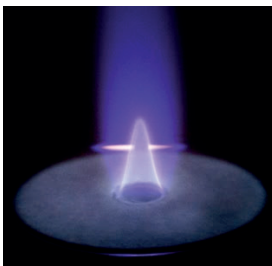
Figure 1: Photograph of a TMI seeded flame with \phi=1.0 using the central jet McKenna burner with laser induced fluorescence of Indium visible.
