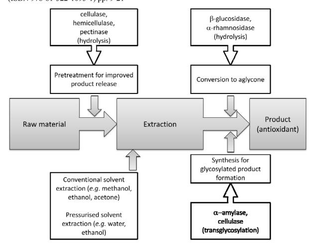
**Figure 2.** Schematic overview of an extraction process to obtain antioxidants with desired glycosylation patterns. The possibilities to use glycoside hydrolases in pretreatment and in conversions to modify the glycosylation are indicated.
