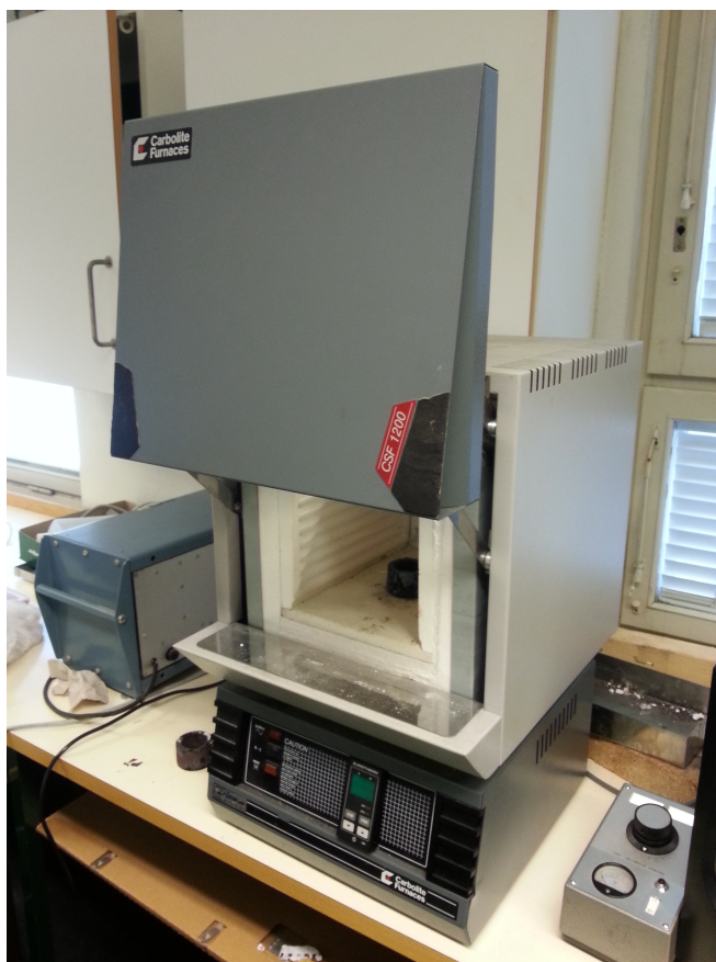
Figure 3.3: The high-temperature furnace equipment used for both oxidation and sublimation experiments.
