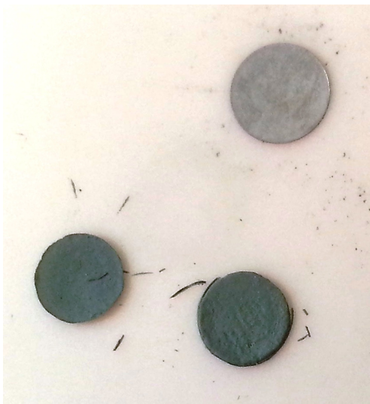
Figure 4.28: Delamination of rolled tungsten foil due to high-temperature oxidation.
