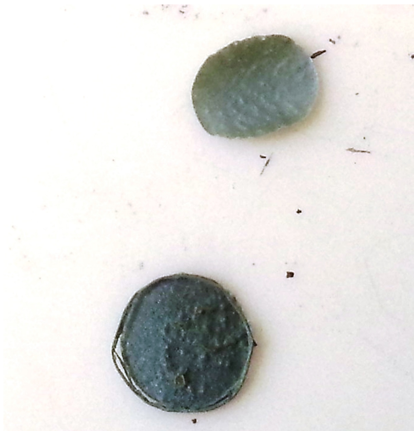
Figure 4.29: Evidence of sublimation of tungsten foil in water vapor containing He at 1075°C for 5 hours.
