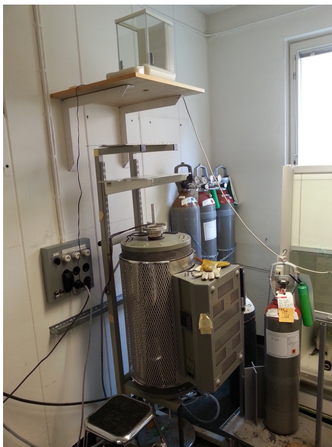
Figure 3.2: The TGA equipment used for both oxidation and sublimation experiments.
