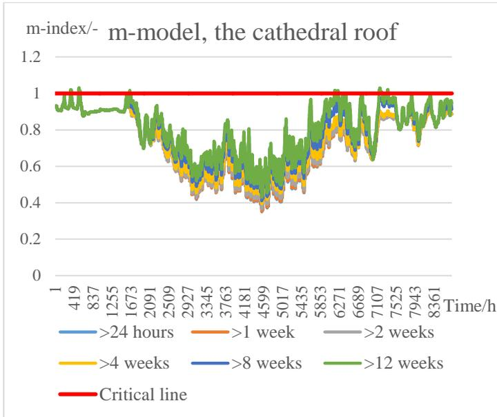
Figure 4.22 m-model results for cathedral roof in Borlänge.
