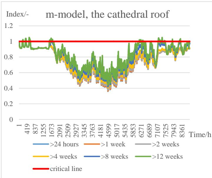
Figure 4.38 M-model, results from the cathedral roof using future climates in Borlänge
