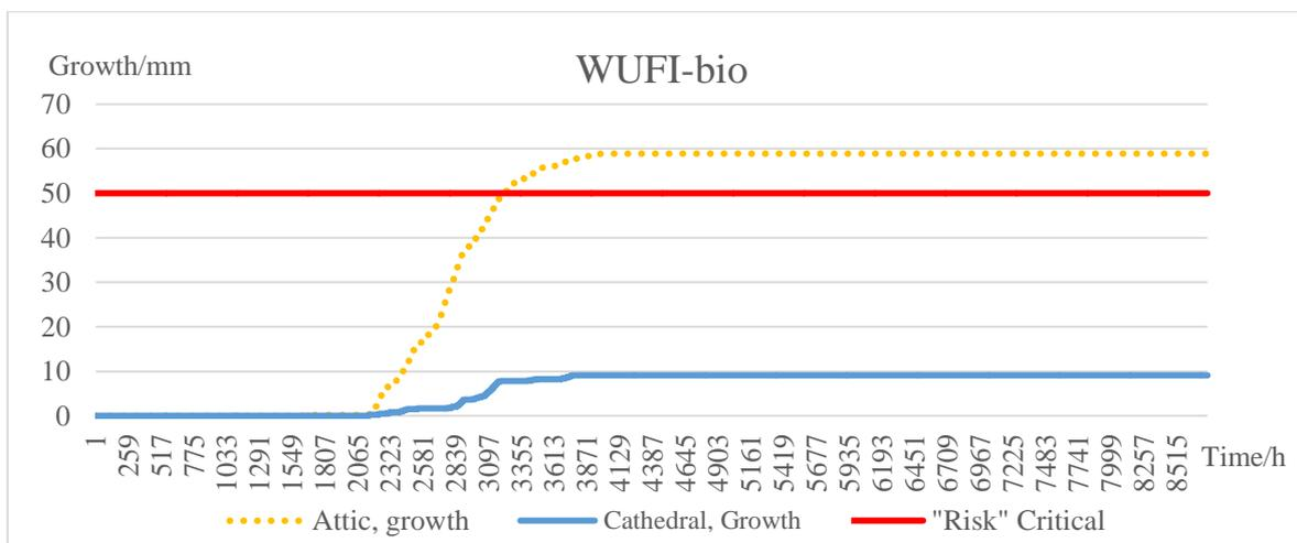
Figure 4.17 WUFI-bio results for attic and cathedral roof in Stockholm. Note that the critical line corresponds the growth, not the index.
