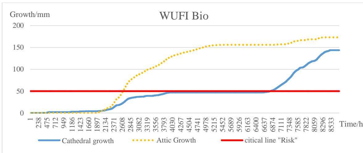
Figure 4.29 WUFI-Bio, a comparison between the cathedral roof and the attic using future climates in Lund. Observe that the critical line is referred to the growth and not the index in WUFI-Bio.
