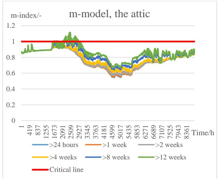
Figure 4.23 m-model results for attic in Borlänge.
