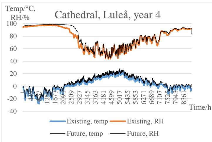
Figure 4.11 RH and temperature in the cathedral roof, for both climates in Luleå.
