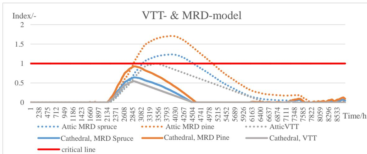
Figure 4.44 VTT- & MRD-model, a comparison between the cathedral roof and the attic using future climates in Luleå
