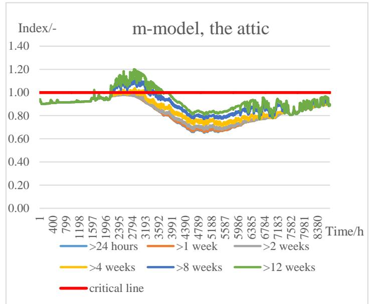
Figure 4.43 M-model, results from the attic using future climates in Luleå
