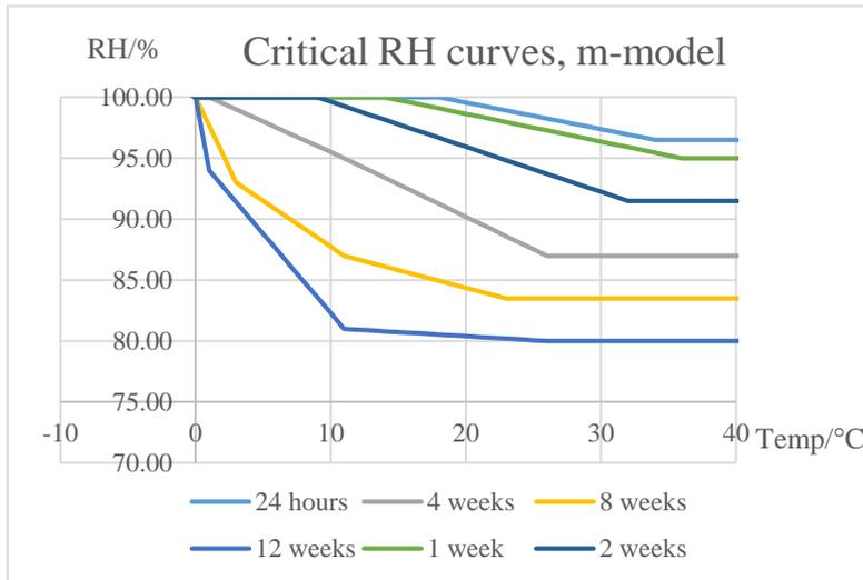
Figure 3.7 Critical moisture levels with safety factor 0.98.
