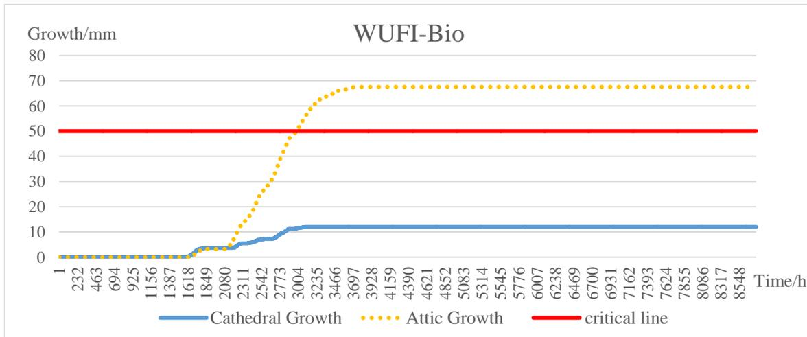
Figure 4.37 WUFI-Bio, a comparison between the cathedral roof and the attic using future climates in Borlänge
