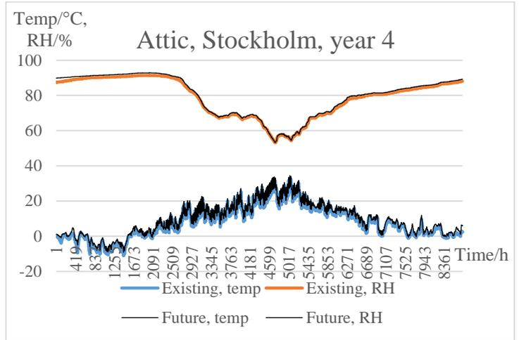
Figure 4.6 RH and temperature in the attic, for both climates in Stockholm.
