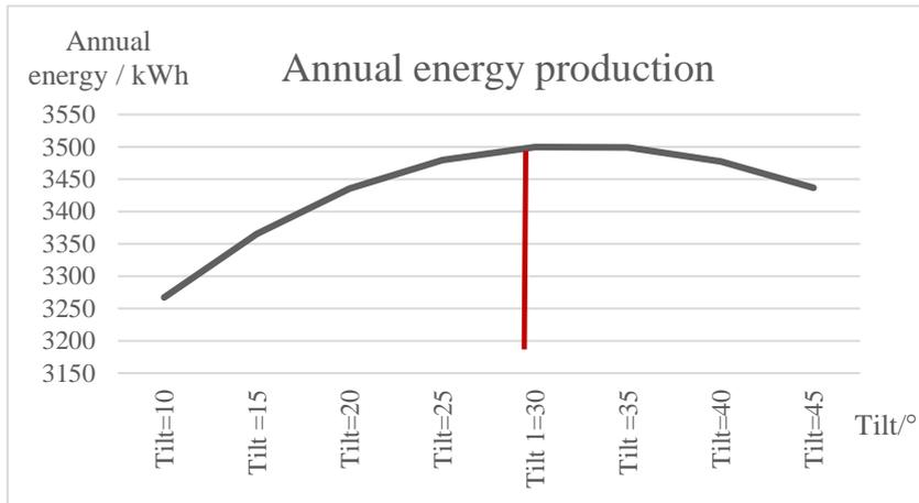
Figure 3.6 Optimal roof tilt with consideration to annual energy output. Simulation made in System Advisor Model (SAM) for location Lund.
