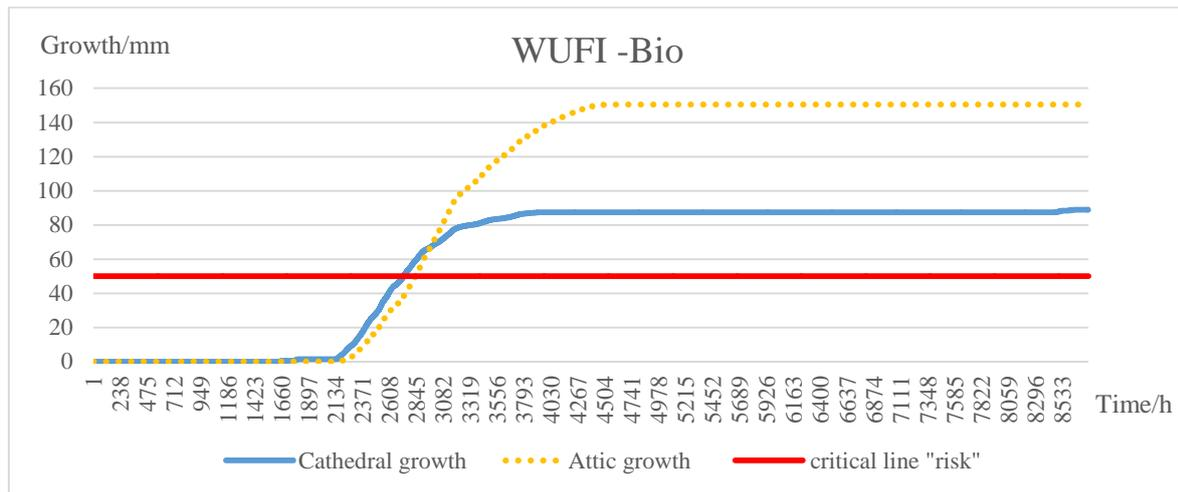
Figure 4.41 WUFI-Bio, a comparison between the cathedral roof and the attic using future climates in Luleå
