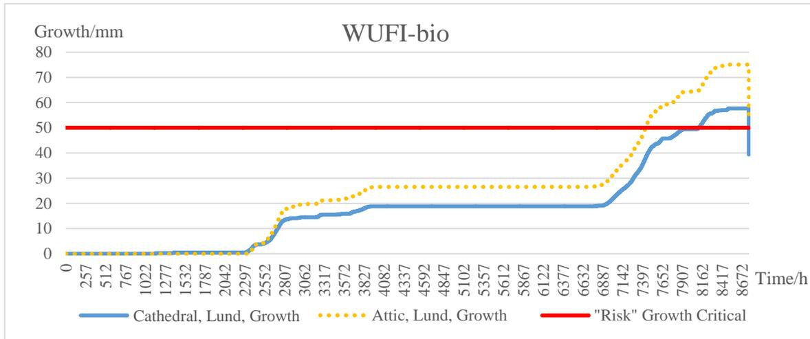
Figure 4.13 WUFI-bio results for attic and cathedral roof in Lund. Note that the critical line corresponds to the growth, not the index.
