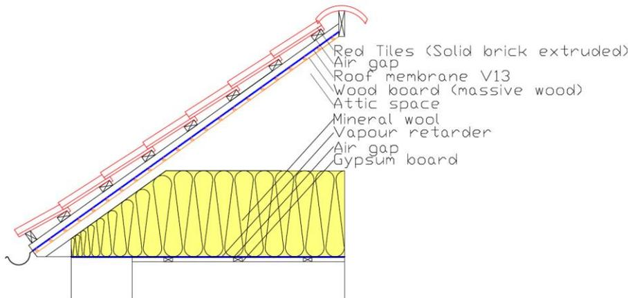
Figure 3.2 An illustration of the attic (drawn in AutoCAD).
