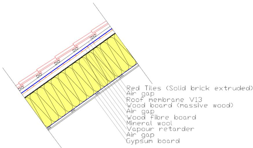
Figure 3.4 An illustration of the cathedral roof (drawn in AutoCAD).
