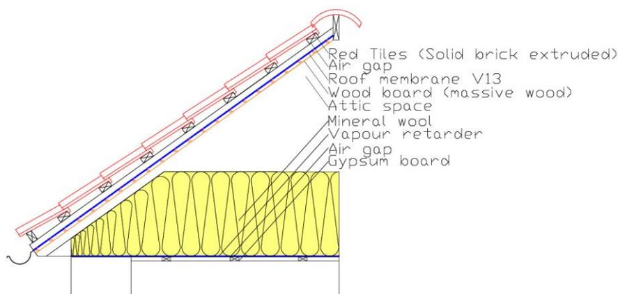
Figure 2.1 Section of an attic and its components (Drawn in AutoCAD)
