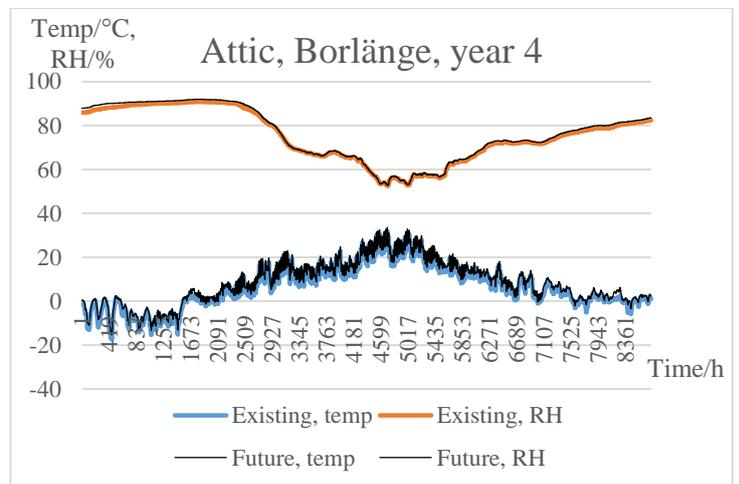
Figure 4.9 RH and temperature in the attic, for both climates in Borlänge.
