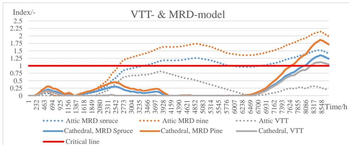
Figure 4.32 VTT- & MRD-model, a comparison between the cathedral roof and the attic using future climates in Lund
