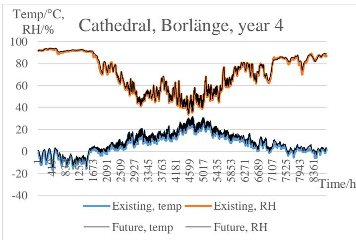
Figure 4.8 RH and temperature in the cathedral roof, for both climates in Borlänge.
