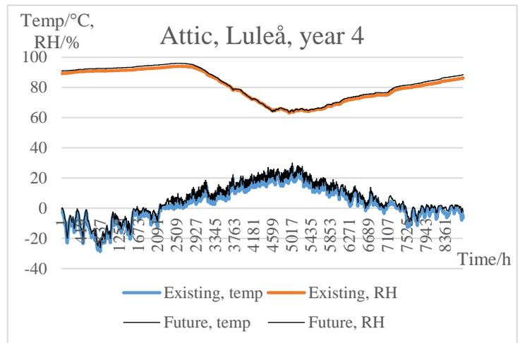
Figure 4.12 RH and temperature in the attic, for both climates in Luleå.
