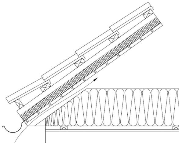
*Figure 2.6 A complementary insulation-layer in the roof reduces the effects of night sky radiation, but also affect the drying out potential during sunny days (drawn in AutoCAD).*
