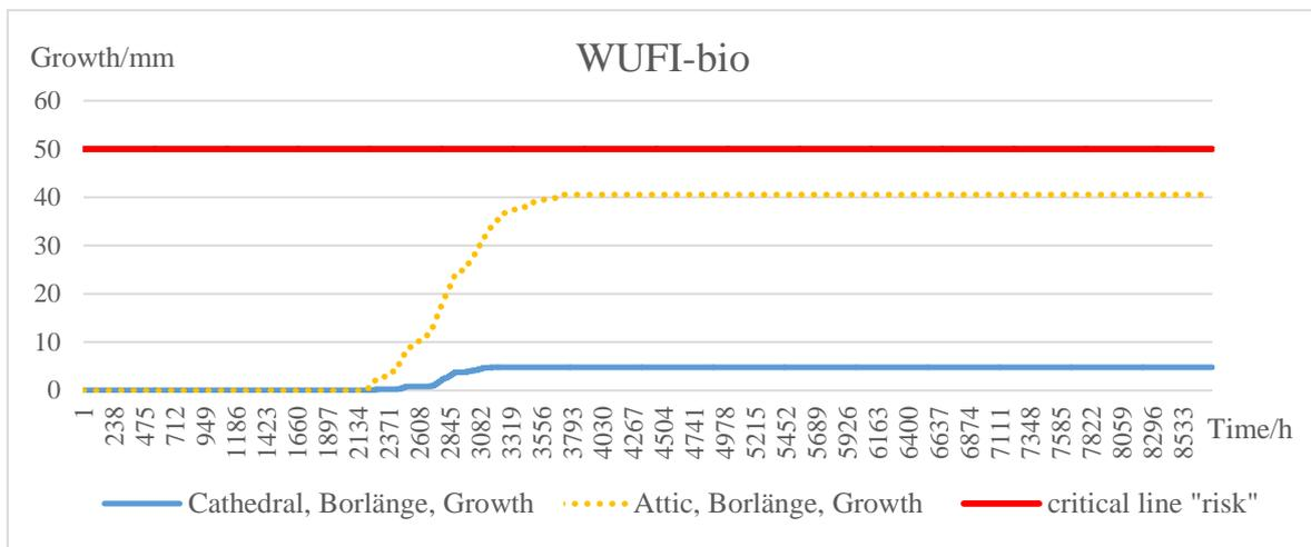
Figure 4.21 WUFI-bio results for attic and cathedral roof in Borlänge. Note that the critical line corresponds the growth, not the index.
