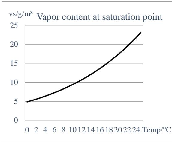
Figure 2.3 Saturated vapour content as a function of temperature
