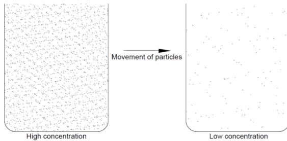
Figure 2.4 Vapour diffusion from high concentration to low concentration (drawn in AutoCAD)
