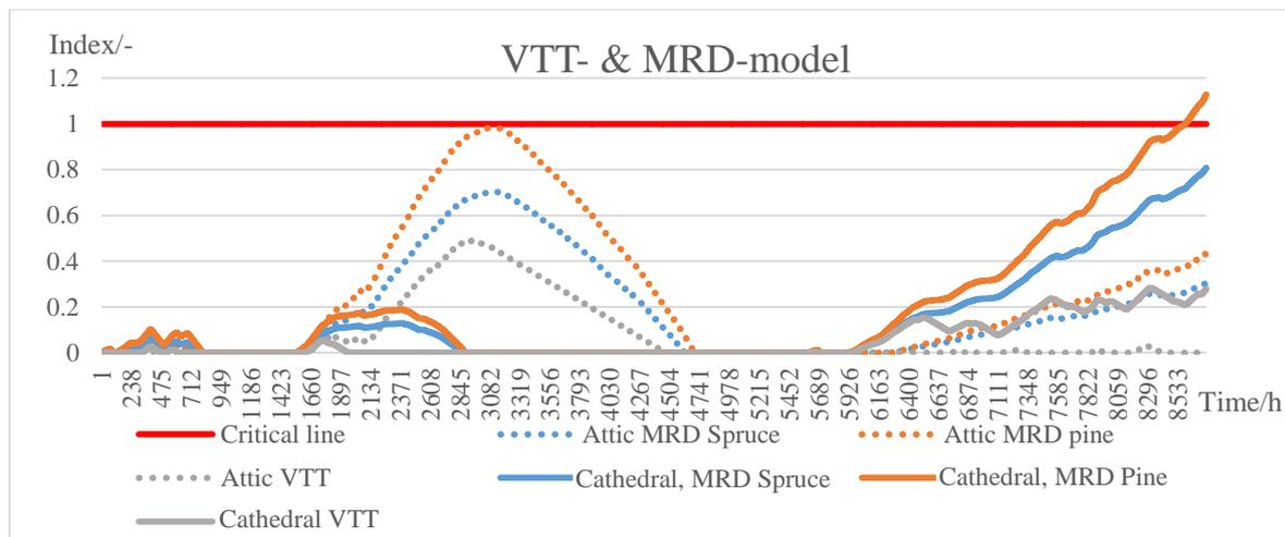
Figure 4.36 VTT- & MRD-model, a comparison between the cathedral roof and the attic using future climates in Stockholm
