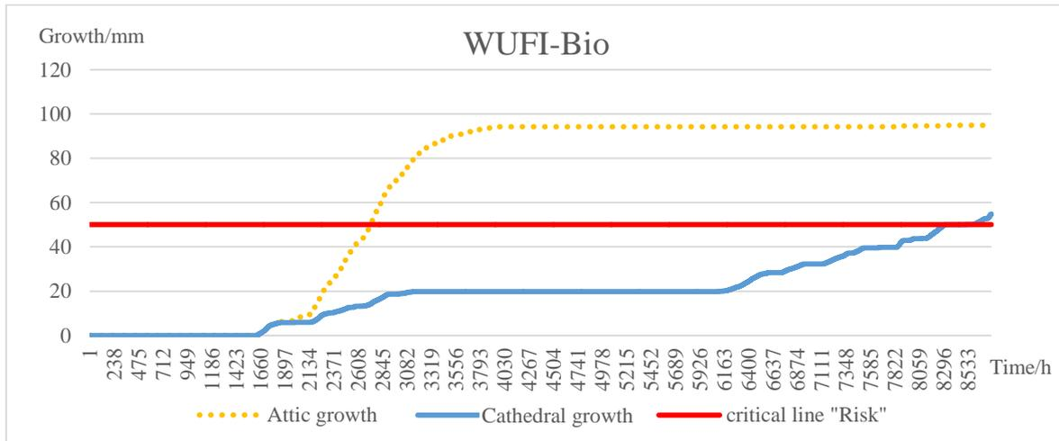
Figure 4.33 WUFI-Bio, a comparison between the cathedral roof and the attic using future climates in Stockholm
