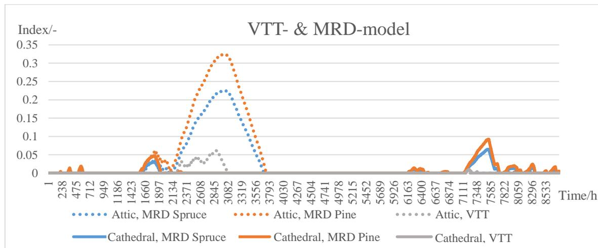
Figure 4.24 Combined graph for the VTT- and MRD-models in Borlänge (Note that the critical line is not visible in this graph)
