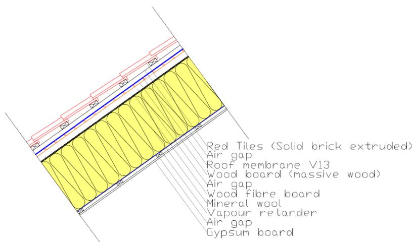
Figure 2.2 Section of a cathedral roof and its components. (Drawn in AutoCAD)
