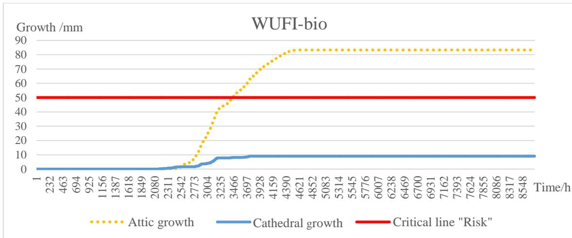
Figure 4.25 WUFI-bio results for attic and cathedral roof in Luleå. Note that the critical line corresponds the growth, not the index.
