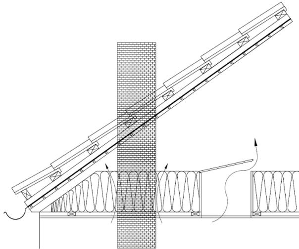
Figure 2.5 Convection through cracks and voids in the system of joints (drawn in AutoCAD)
