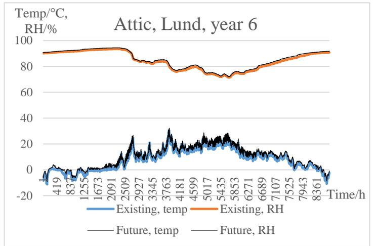
Figure 4.3 RH and temperature in the attic, for both climates in Lund.
