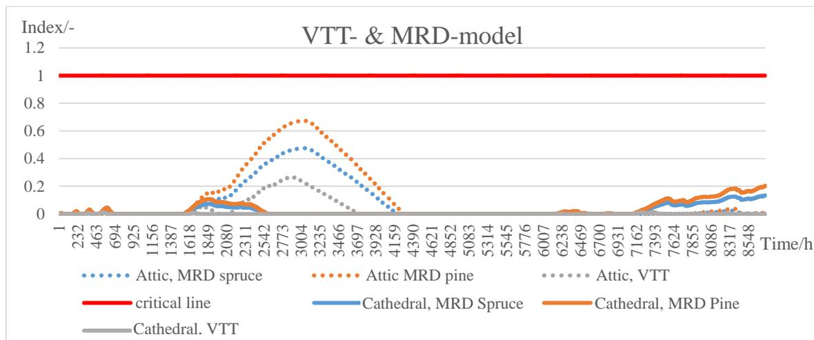
Figure 4.40 VTT- & MRD-model, a comparison between the cathedral roof and the attic using future climates in Borlänge
