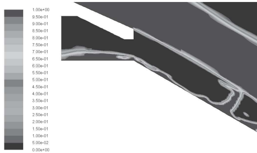
FIGURE 6.17: Water in the aerator (2D- 1500m^3/s )
