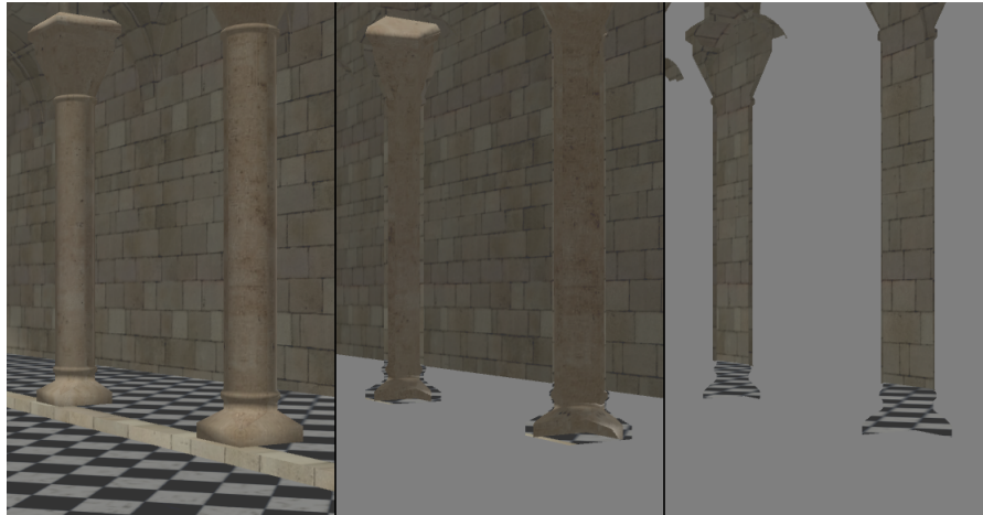
Figure 1.3: Demonstration of depth peeling. Scene rendered with a G-buffer with three layers. First layer is shown to the left, second layer in the middle and third layer to the right. Each layer contains information that was obscured in the previous layer.
