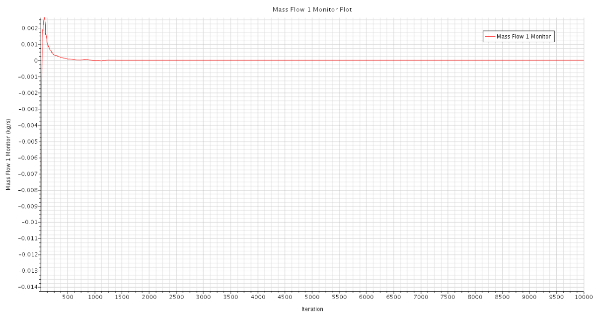
Figure A.1: Report plot of the difference between the mass flow at inlet and outlet
