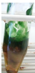
Figure 14 PL40 oil mixed with 20% (v/w oil) water and 50 \mu L of 5M NaOH. Due to the high viscosity of PL40 oil, the base did not mix homogeneously, leading to a high pH at the top. The green colour is likely caused by phenolic acids present in oat oil, which are known to display a green colour when the pH is high (Doehlert et al. 2009).
