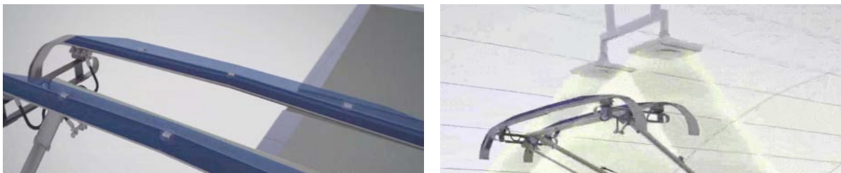
Figur 17: Sensorsystem i "Intelligent carbon for pantograph", (Schunk, 2013)
