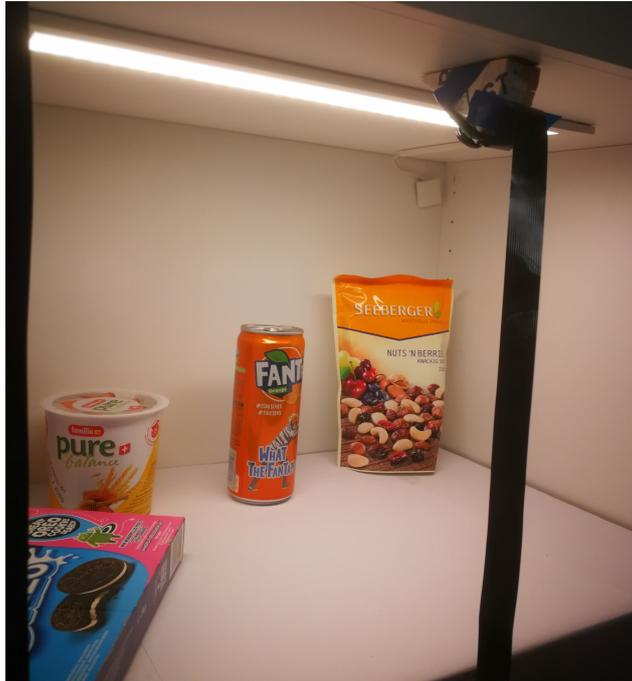
Figure 4: Setup for the data gathering process. A Raspberry Pi camera was mounted inside the shelf and a majority of the training data was captured this way, to mimic the run-time environment as close as possible.
