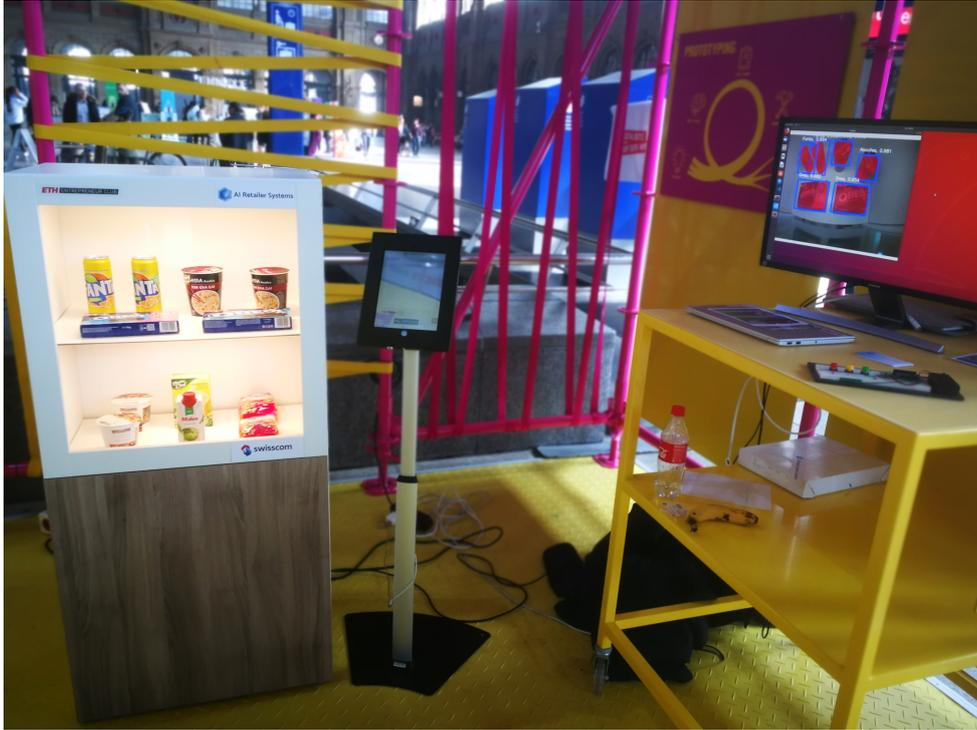
Figure 10: The complete prototype with the shelf with products, the front-end application running on the iPad in the stand as well as a visualization of the model running live on the big PC screen.
