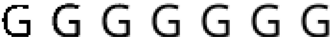
Figure 1.3: A glyph rasterized at 24px with different subpixel sampling rate. From left to right 1,  $(2 \times 2)$ ,  $(4 \times 4)$ ,  $(8 \times 8)$ ,  $(16 \times 16)$ ,  $(32 \times 32)$ ,  $(64 \times 64)$  samples per pixel.
