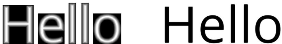
**Figure 3.4:** (Left) A set of quads with SDF textures. (Right) The quads on the left rendered with an SDF shader.
