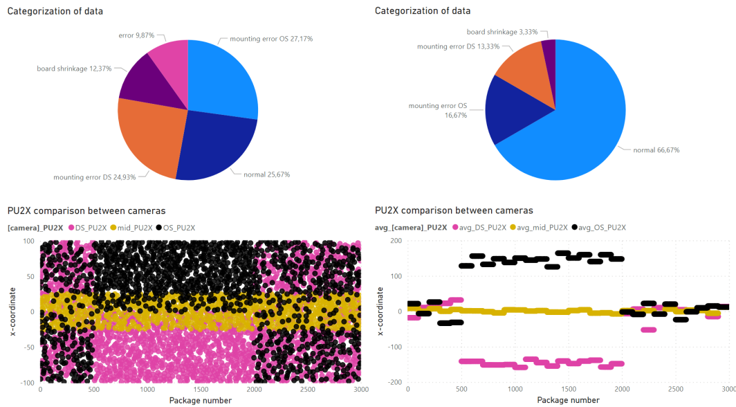
Figure 4.10: The data categorization of the partly implemented prototype. Visualizations of single sensor values are presented on the left side and the average of each 100 rows of data are presented on the right side.
