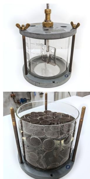
Figure 3.2. Empty reactor (top), reactor with carriers (bottom)
