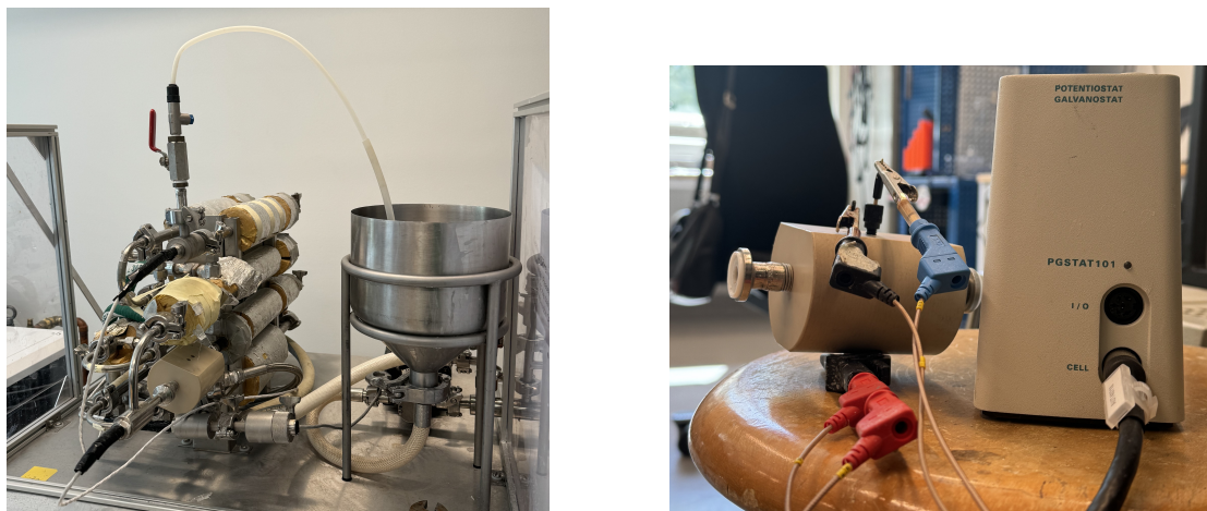
Figure 8: Close ups of setup. To the left, close up of attached test chamber, isolated piping and electrolyte tank. To the right, attachment of electrodes to potentiostat, not attached to corrosion testing machine. Counter electrode (black), reference electrode (blue) and working electrode (red).
