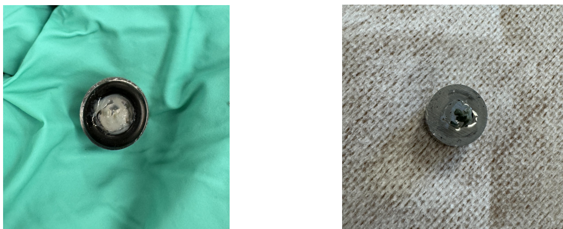
Figure 29: Fouled samples, left from processing at 1000 ppm, 30 °C and 96 g/950 mL milk and right from 1000 ppm, 80 °C and 96 g/950 mL.
