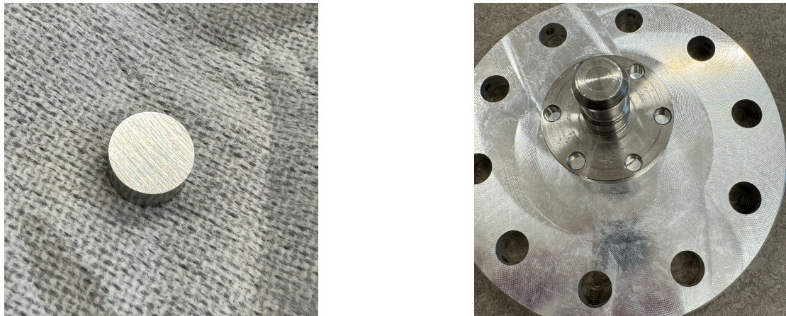
Figure 11: Grinded sample and sample holder used to grind samples.
