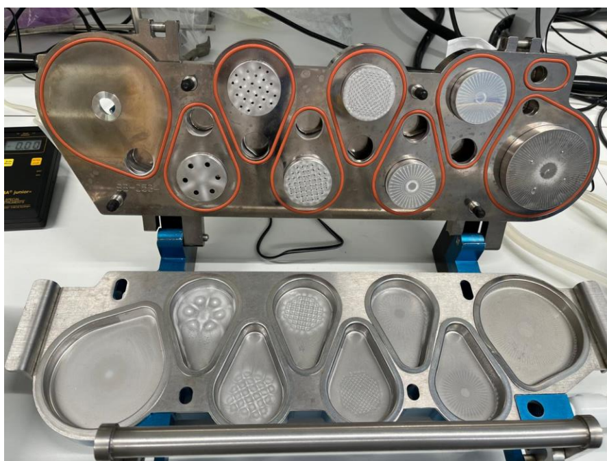
Figure 34: NGI stages after using Trehalose_Leucine_BSA_02 with RS01 inhaler.
