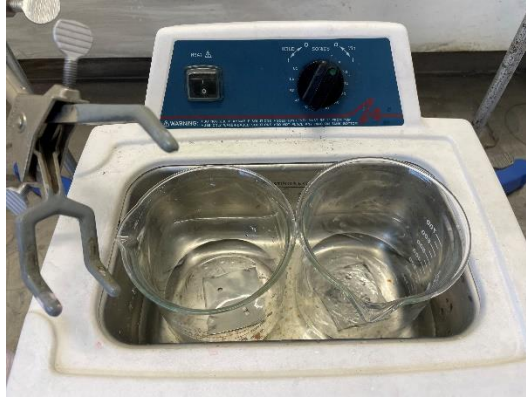
Figure 6: Ethanol(left) and isopropanol (right) cleaning liquid in ultrasonic machine.
