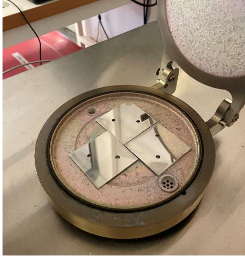
Figure 8: Three samples were placed in the reaction chamber to await deposition for Savannah 100 ALD machine.
