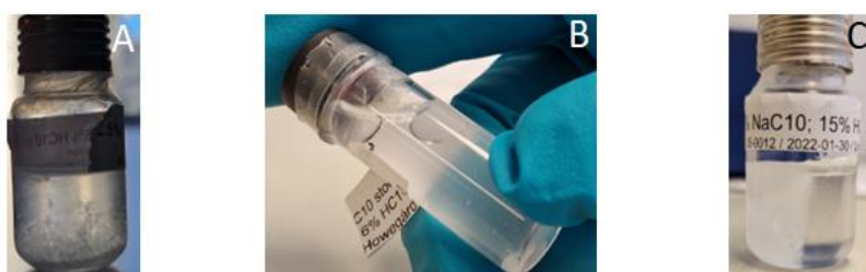
Figure 17: Shows what happened to solid crystals, most obviously observed for samples that contained high fractions capric acid, when they are heated to 37°C. Within a short period of time the crystals melt and form droplets of oil that floats on the top, as shown in Figure B. Figure C shows an example of what those samples could look like after a week at 37°C.
