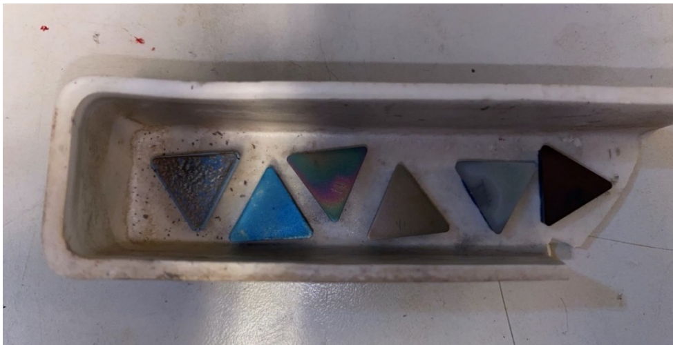
Figure 4-3 Furnace samples placed from the left: C1, C2, C3, C4, TiN and TiAlN, after 1 hour in 800 °C.
