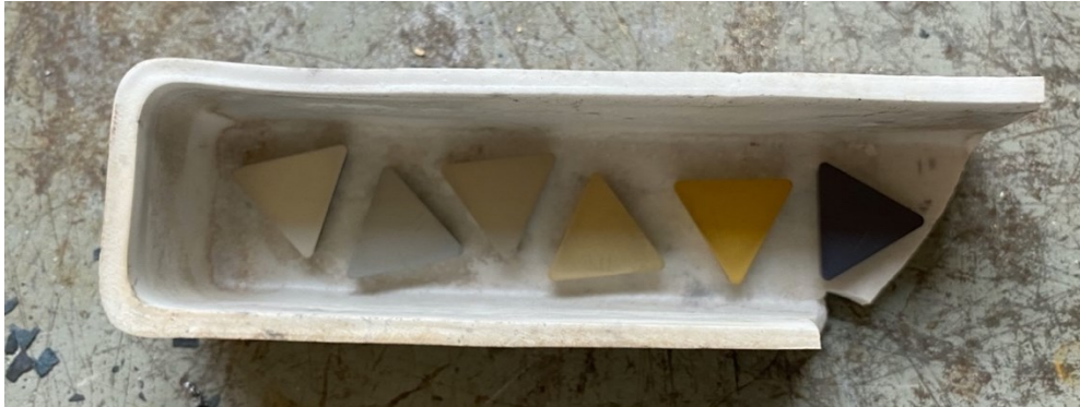
Figure 3-2 Coating C1, C2, C3, C4, TiN, and TiAlN before being exposed to 800 °C for 1 hour.
