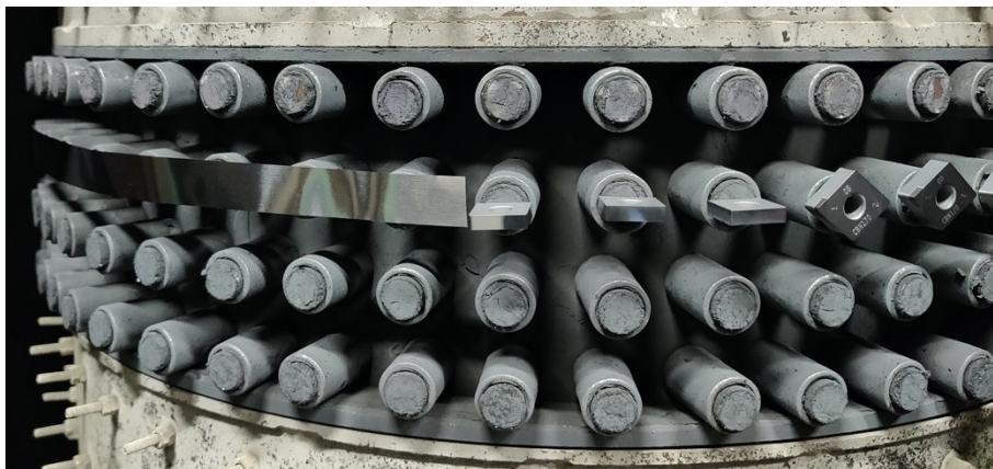
Figure 3-1 Foil and tools mounted at a specific level in the PVD furnace.
