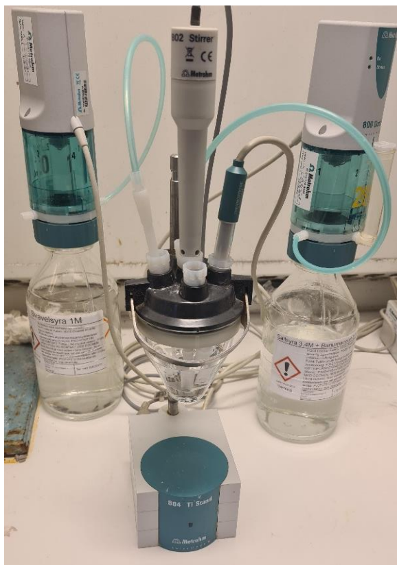
Figure 2: Equipment used in the thermometric titration (Metrohm 859 Titrotherm)
